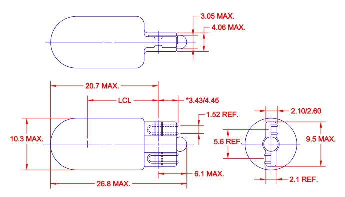
\*TO BE MEASURED ON LONGEST SIDE ONLY WITH THE WIRE IN INTIMATE CONTACT WITH THE BOTTOM OF THE GLASS WEDGE.
